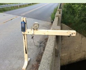
A hand-crafted bridge board allows FBE to conduct flow monitoring in non-wadeable rivers
