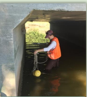
Lauren deploying a data sonde in Spruce Creek, Kittery, ME
